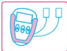
Connect the main unit with electrodes using the Y-cable
